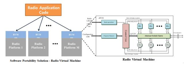
Figure 7. Concept of the Radio Virtual Machine
