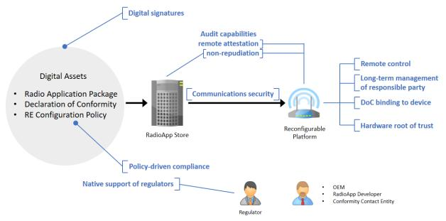
Figure 6: Security measures for the ETSI Software Reconfiguration framework
