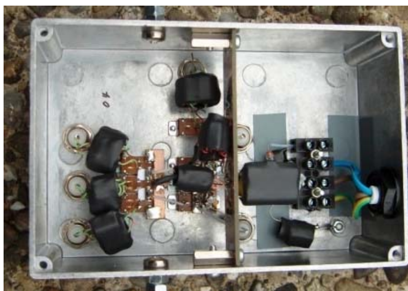
Figure 19: Photograph of Coupler, Case Opened
