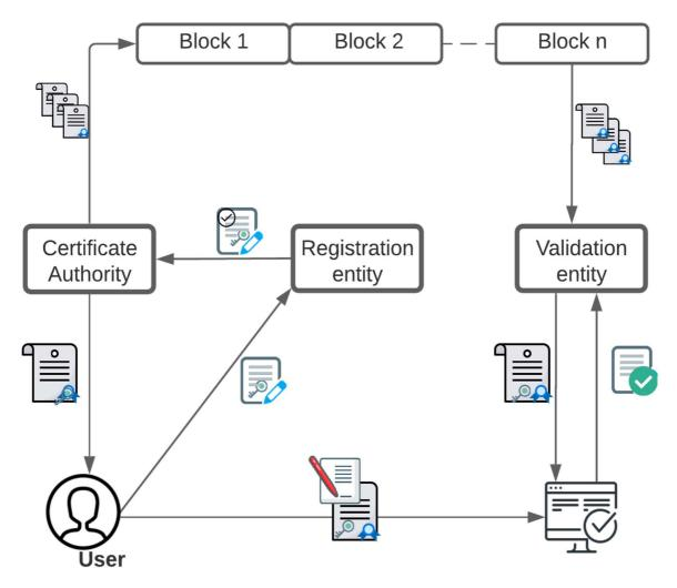
Figure 7-1: Example of PDL based Certificate Authority
