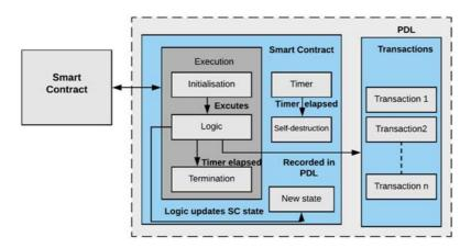
Figure 6-3: Reference Architecture of a Smart Contract with contract chaining
