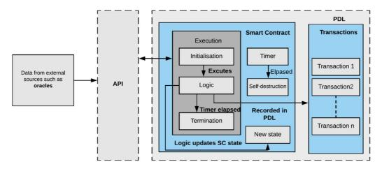
Figure 6-2: Reference Architecture of a Smart Contract without contract chaining
