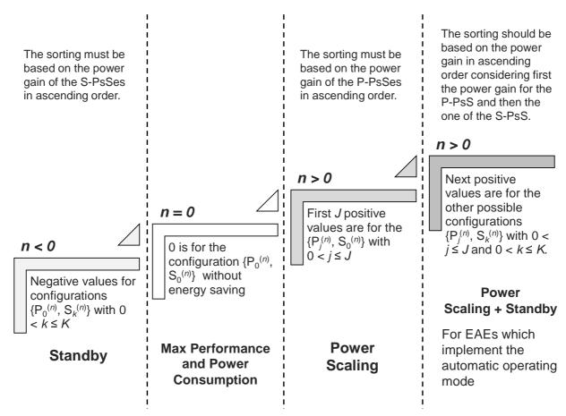
Figure 2: EAS identification mapping
