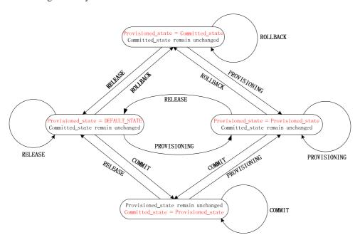
Figure B.2: Logical Entity State Transition Diagram
