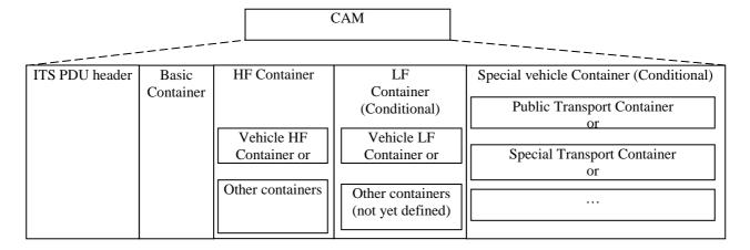
Figure 4: General structure of a CAM
